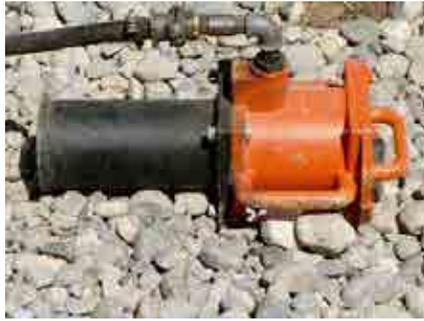
Fig. 4 – Pneumatic pile driver GR40 with guide bush IPE 100
